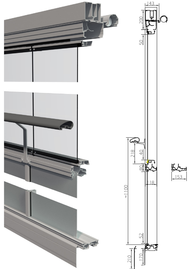
Design Air. Cross section and drawing from the side.
